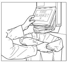
Open the front, dampen, and slide the blanket into the asbestos waste bag
