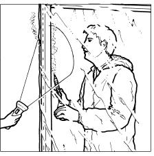
Test the enclosure for leaks with a smoke test
