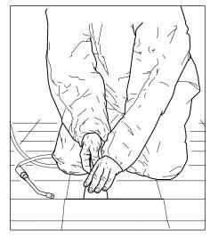
Spray water under the tiles to suppress dust as you lift them gently, avoiding breakage
